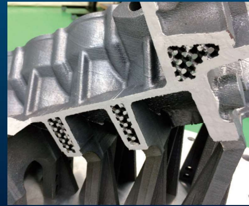
V8 engine block with lattice structure
